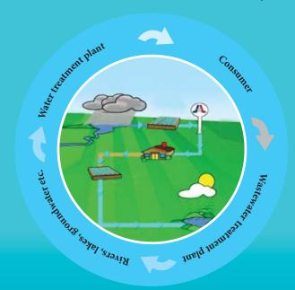
To ensure public health in a city it is important to maintain the wastewater treatment cycle. Wastewater must be treated in wastewater treatment plants before being discharged into rivers, lakes and groundwater from where, drinking water will be collected and then processed in water treatment plants before being delivered to the consumer. Only a well-functioning water treatment cycle can ensure public health and well being in a city.
